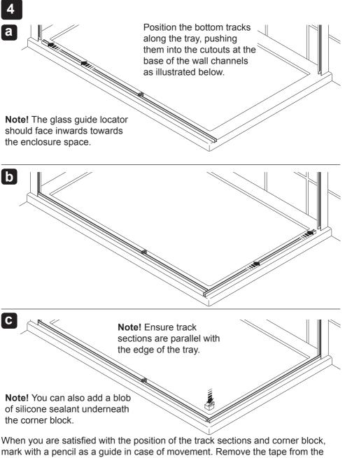
underside of the side panel track and stick into place. As an aid during installation it is also advisable to use additional tape to prevent movement. This can be removed once the glass panels are installed and beaded.
