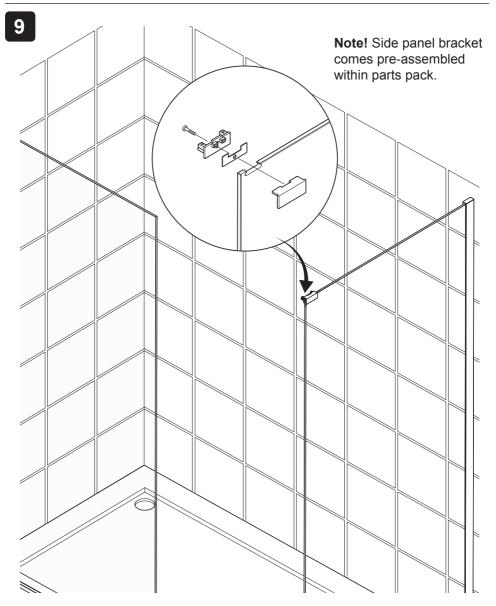
(a) Secure the side panel bracket using screw.
