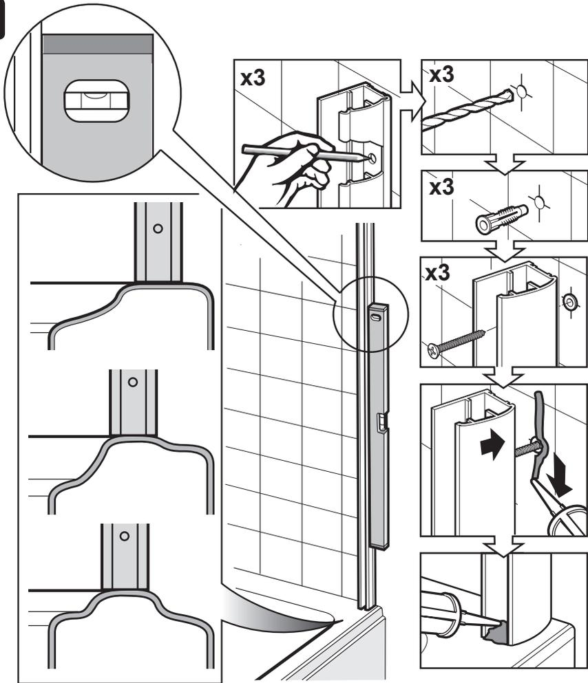
(a) Position the wall channel on the wall. Using a spirit level make sure that it is upright.
