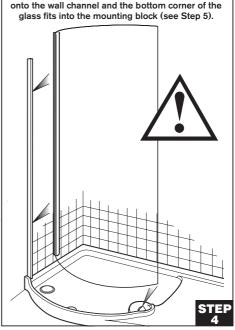
Carefully lift the glass into place. The jamb fits
