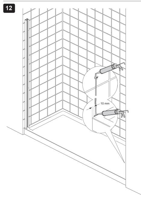
(a) Apply silicone sealant along the length of the wall and at the bottom where the wall channel will be placed.
