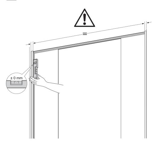
(a) Centralise the door frame within the wall channels, making sure that the door frame is square.
