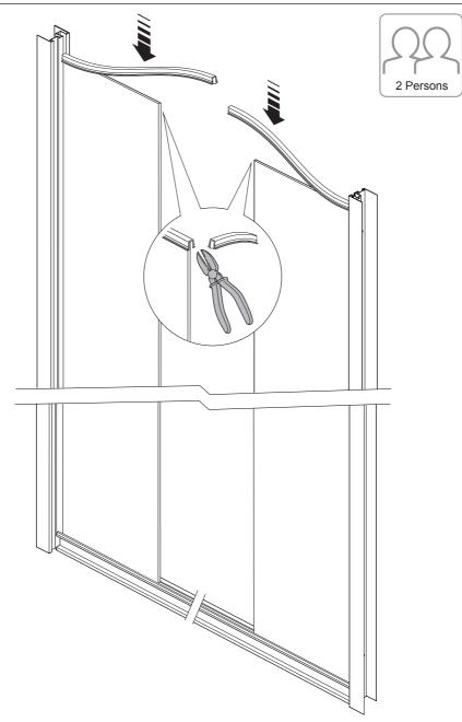
(a) Install the seals to the top of the panels as shown above and cut to length, leaving 5 mm extra to allow for shrinkage.
