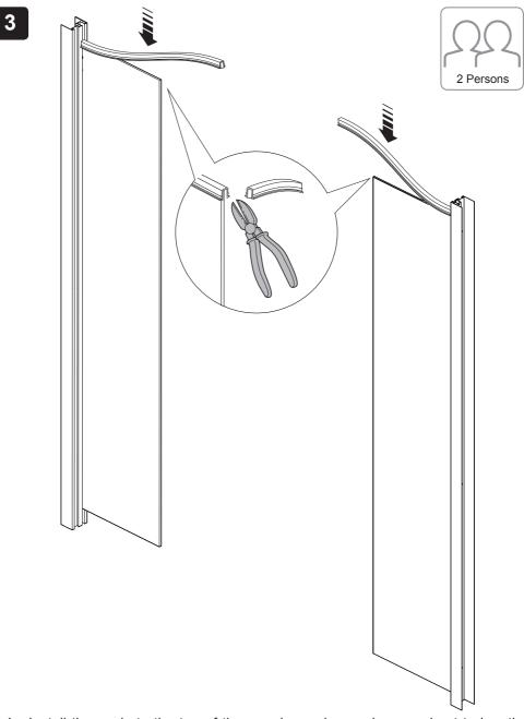
(a) Install the seals to the top of the panels as shown above and cut to length, leaving 5 mm extra to allow for shrinkage.
