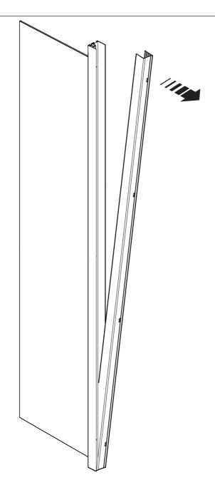
(a) Remove the wall channel from the panel.
