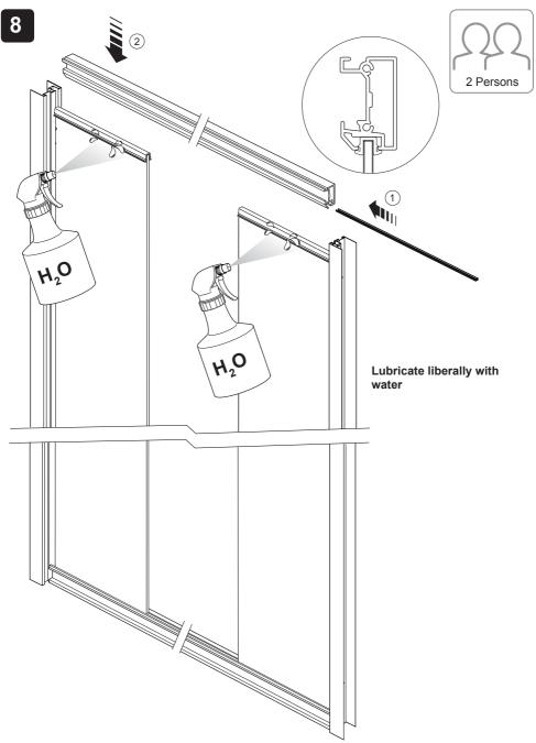
(a) Slide the track infil into the middle of the channel and lower the track onto the seal.
