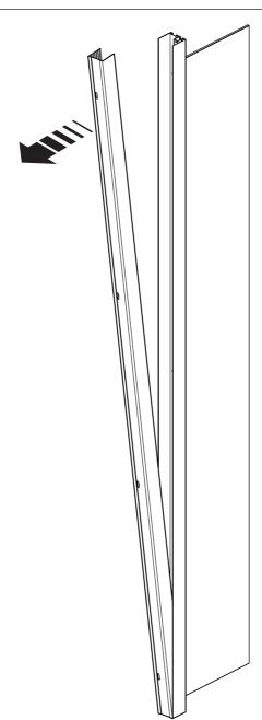
(a) Remove the wall channel.
