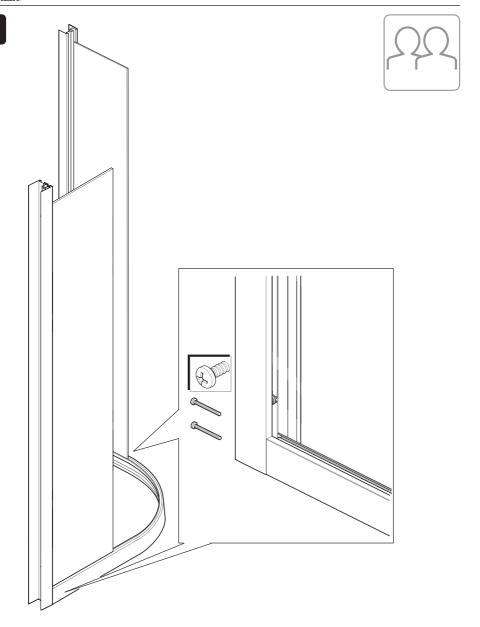
(a) Install the screws to both sides to secure the assembly.
