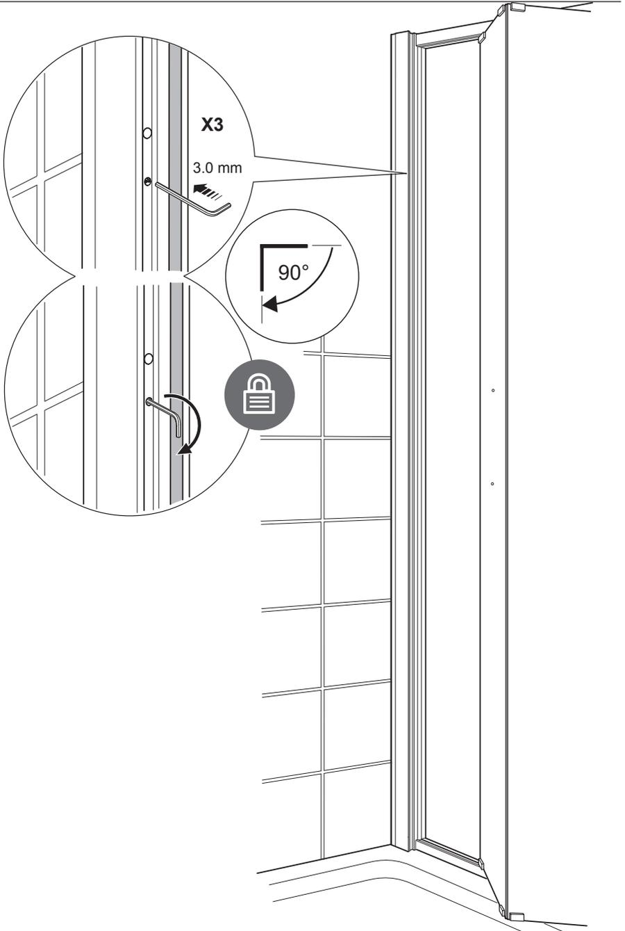
(a) Using the 3.0 mm hexagonal wrench (supplied), turn through 90° clockwise in three locations to lock the door frame in position.
