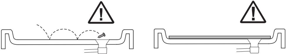
**Note!** Cover the tray waste to prevent the loss of small parts.
