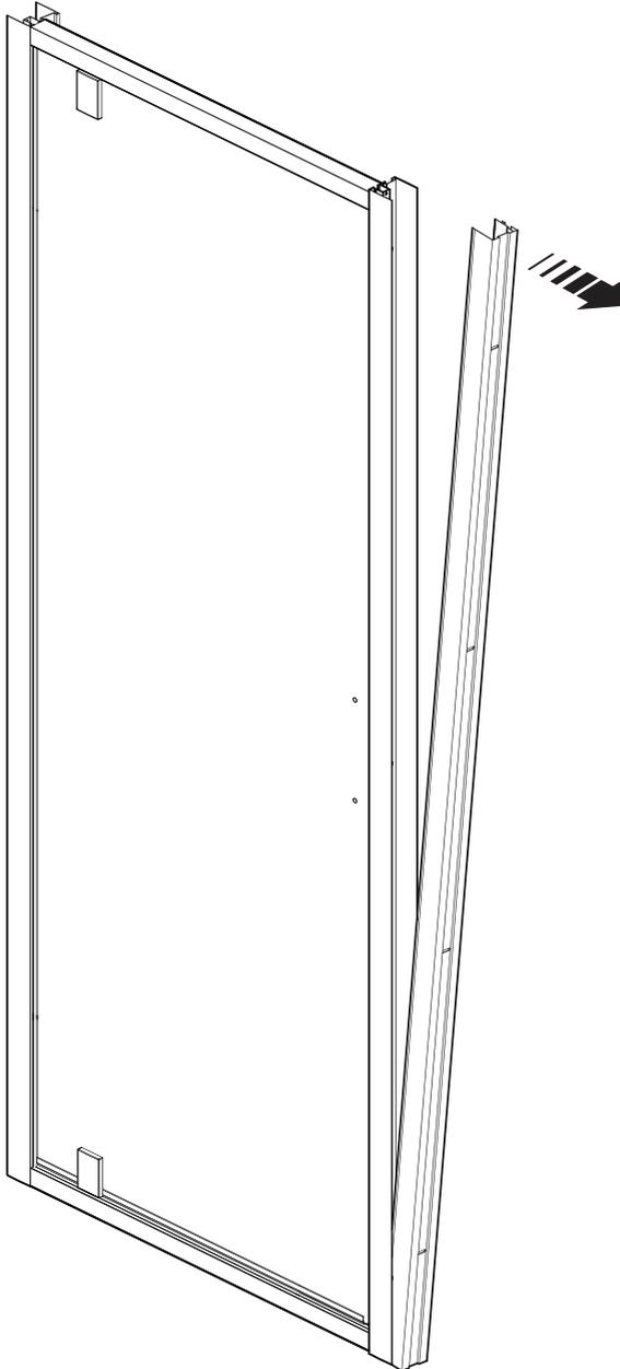
(a) Remove the wall channel from the door.
