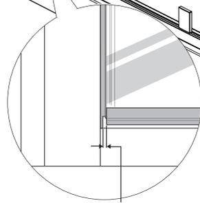
**Note!** Adjust door to minimise seal gap
