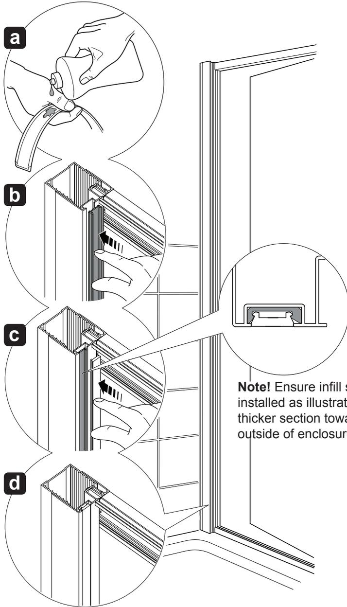
**Note!** Ensure infill strip is installed as illustrated with thicker section towards outside of enclosure.
