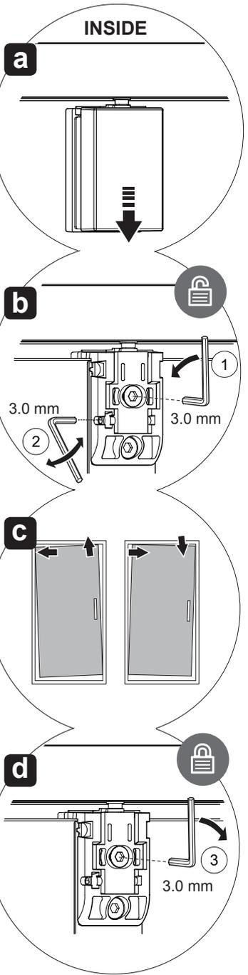
(b) If the door is out of square, adjust as shown above.
