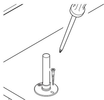
5. Offer the Ceiling-Fed Arm to the brass pipe and determine the showering height required. Push or pull the brass pipe using a twisting motion to adjust the height. Check the height is correct and use a 15 mm pipe cutter to cut the pipe to the desired length. **Note!** Cut the brass pipe at least 30 mm above the ceiling mount plate to allow room to fit the olive, nut and elbow.
