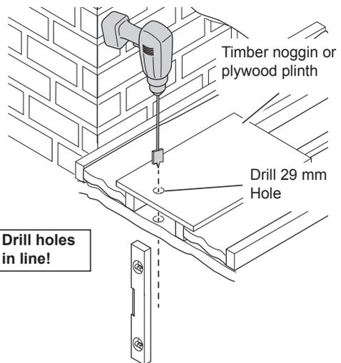
2. Drill a 29 mm hole through the ceiling and the wooden support. Ensure the two holes drilled are directly in line or the ceiling pipework will be at an angle.
