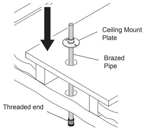
4. Centralise the brass pipe in the hole then screw the ceiling mount plate to the wooden support.
