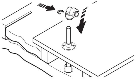
10. Connect the shower control outlet pipework to the elbow. Fit an isolating valve between the shower control outlet and the elbow to enable easy maintenance. (Pipe and isolating valve not supplied). Lock pipe to elbow using clip supplied. Follow manufacturers guidelines for fitting alternative push-fit connections and flexible pipework.
