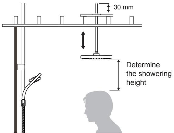
6. Secure the brass pipe to the ceiling mount plate with the olive and 1/2" BSP nut. **Note!** This is not a water tight connection, tighten sufficiently to clamp the pipe in place.
