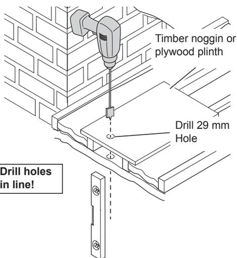
2. Drill a 29 mm hole through the ceiling and the wooden support. Ensure the two holes drilled are directly in line or the ceiling pipework will be at an angle.
