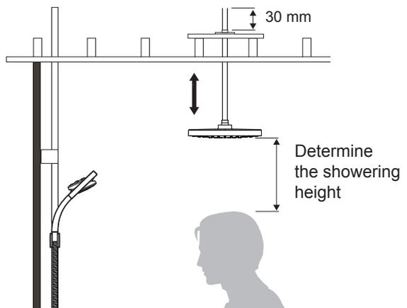
6. Secure the brass pipe to the ceiling mount plate with the olive and 1/2" BSP nut. **Note!** This is not a water tight connection, tighten sufficiently to clamp the pipe in place.
