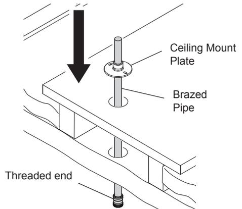
4. Centralise the brass pipe in the hole then screw the ceiling mount plate to the wooden support.
