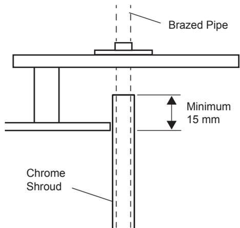
8. Push the chrome shroud into the ceiling plate then slide the chrome shroud over the threaded end of the brass pipe and up through the hole until the ceiling plate is secured in the hole and the ceiling plate is flat against the ceiling.
