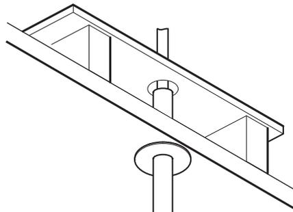
11. Ensure pipework is thoroughly flushed through before fitting the deluge head.
