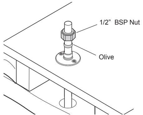
7. Offer the chrome shroud to the brass pipe and determine the length required to allow the shroud to conceal the brass pipe and protrude into the ceiling space a minimum of 15 mm. Use a pipe cutter to cut the shroud to the desired length.
