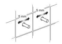
**5.** Fit the installation template over the inlet pipes and mark the positions of the 4 wall bracket fixing holes.
