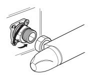
**15.** Loosely screw the concealing plates onto the offset connectors **Important!** Do not fully tighten at this stage.
