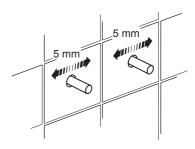
4. Important! Make sure that there is still horizontal movement on the inlet pipes, if not, continue with the installation making sure that you complete section: 'Installation with Fixed Pipework' when instructed, this will avoid cracking tiles.
