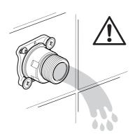
**14.** Offer the bar valve up to the offset connectors, and if necessary, rotate the connectors anti-clockwise to adjust the centres.
