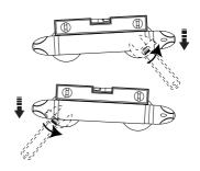
Tighten the concealing plates until they are flush with the finished wall.
