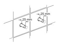
Drill the 4 holes for the wall brackets with a 6 mm drill and insert the wall plugs (some wall structures may require alternative fixings, not supplied).
