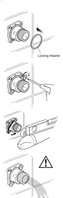
**6.** Tighten the concealing plates until they are flush with the finished wall.
