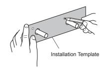
6. Mark the pipe distance  $25 \pm 5$  mm from the finished wall and cut to length.
