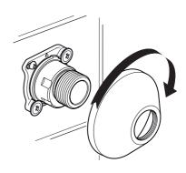
7. Make sure that the sealing washer/filter is fitted in the correct orientation, offer the bar valve up to the offset connectors and tighten the nuts.
