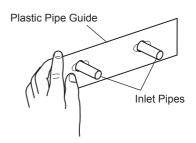
3. Leave the plastic pipe guide in place and finish the wall.
