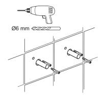
Fit the wall brackets and olives onto the inlet pipes and loosely fit the nuts.
