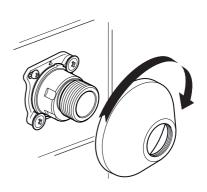
**16.** Make sure that the sealing washer/filter is fitted in the correct orientation, offer the bar valve up to the offset connectors and tighten the nuts.
