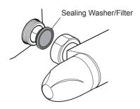
**8.** Turn on the hot and cold water supplies and check for leaks.
