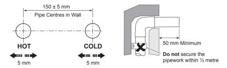
1. Install the pipework making sure that it is level and set the correct distance apart  $(150 \pm 5 \text{ mm})$ .
