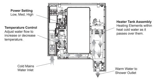
Hot water is produced by passing cold water through a heating tank.
