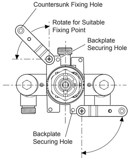
**Note!** Securing Brackets shown in preferred position to allow the Compression Nuts to be tightened.
