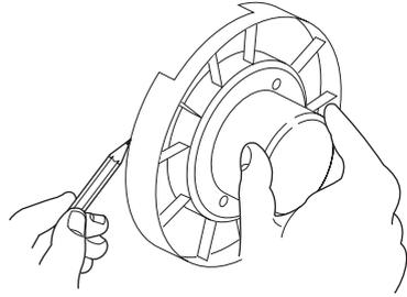
**1.2** Remove the two Shroud Screws (retain for later use) and remove the Mixer from the Building-in Shroud.
