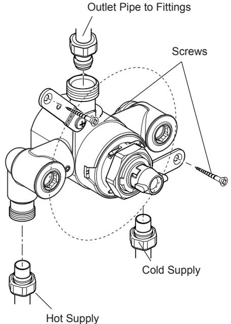
**1.15** Attach the Building-in Shroud to the Mixer using the two Shroud Screws removed earlier.
