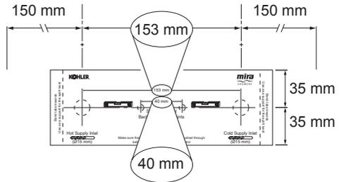
**2.3** For solid walls drill the holes for the Backplate with a 6 mm drill and insert the Wall Plugs (supplied). For other types of wall structure alternative fixings may be required (not supplied).
