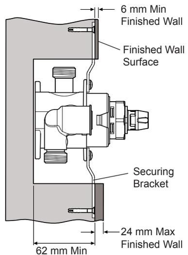
**1.7** Remove the plasterboard and/or brick work to a minimum depth of 62 mm.
