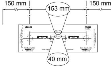
1.2 For solid walls drill the holes for the Backplate with a 6 mm drill and insert the Wall Plugs (supplied). For other types of wall structure alternative fixings may be required (not supplied).
