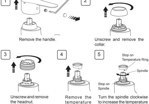
to increase the temperature and anticlockwise to decrease the temperature. Refit the temperature control ring making sure the stop is against the stop on the spindle. Repeat until you have reduced the temperature to your required
