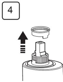
Remove the temperature control ring.
