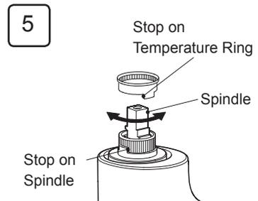
Turn the spindle clockwise to increase the temperature and anticlockwise to decrease the temperature. Refit the temperature control ring making sure the stop is against the stop on the spindle. Repeat until you have reduced the temperature to your required setting.
