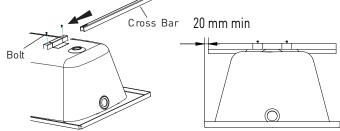
3. Install the feet onto the cross bars and secure them in position with the nuts.
