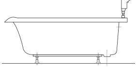
10. If required, mark the positions of the holes for the taps and drill with a suitable tool.
