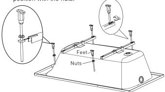
4. Install the end of the steel bars onto the plastic parts.
