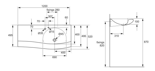
All measurements shown are in millimetres. Sizes are approximate.
