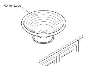
12. Carefully place the vessel in position.
