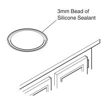
**11.** Apply a 3 mm bead of silicone sealant around the edge of the cutout hole. Apply the sealant approximately 6 mm away from the cutout hole edge.
