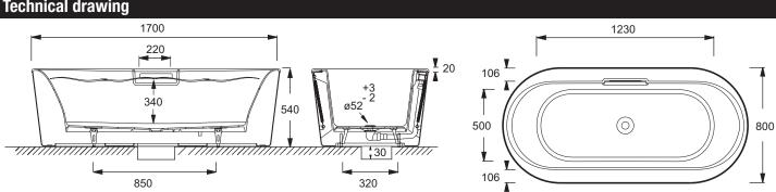
Product Specification: Freestanding bath 170 x 80 cm. 6D063. Collection: VOLUTE. Dimensions: 170 x 80. Weight: 150 kg. Material: Cast iron. Installation: Floor-standing. Volume: 216/146. Shape: Oval. Incl. factory-assembled reinforced acrylic panel and built-in waste 6D064. Trap and connection kit E75307. To install waste, lay trench 3 cm deep in the floor or build platform...
