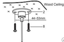
For wood ceiling, install the screws(8) at the proper position in the ceiling according to the marked dimensions.
