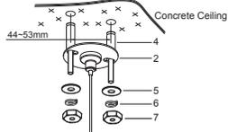
For concrete ceiling, drill eight holes(Ø8mm) at the proper position in the concrete ceiling according to the marked dimensions and expansion screw's(4) diameter. Hammer expansion screws into the holes(Ø8mm). Secure the fix bases(2), the washers(5) and the locking gaskets(6) on the concrete ceiling with the nuts(7).
