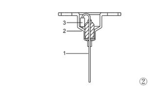
Make sure the end(3) of the stainless wire(1) is in the fix base(2) before install as shown to the figure.
