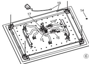
Before install the rainhead(9), install regulator(14) if needed. Remove the shower connectors(15, 16), hoses and washers, install regulators as the figure shown. Reinstall the washers, hoses and shower connectors.
