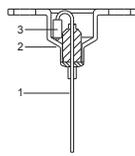
Make sure the end(3) of the stainless wire(1) is in the fix base(2) before install as shown to the figure.
