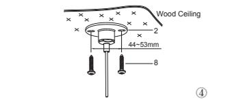
For wood ceiling, install the screws(8) at the proper position in the ceiling according to the marked dimensions.
