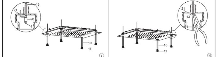
Upon connecting, one hand push the rainhead upwards, another hand drag the stainless wire gently, make sure the rainhead against the suspended ceiling, the stainless wire is perfectly straight. Insert the spare wire into the clip(20), and insert the stainless wire into the hole(21) as shown in the figure. Press the cap with O-ring.
