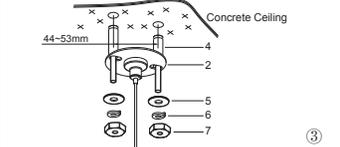
For concrete ceiling, drill eight holes(Ø8mm) at the proper position in the concrete ceiling according to the marked dimensions and expansion screw's(4) diameter. Hammer expansion screws into the holes(Ø8mm). Secure the fix bases(2), the washers(5) and the locking gaskets(6) on the concrete ceiling with the nuts(7).
