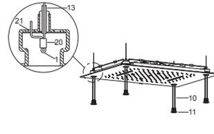
Upon connecting, one hand push the rainhead upwards, another hand drag the stainless wire gently, make sure the rainhead against the suspended ceiling, the stainless wire is perfectly straight. Insert the spare wire into the clip(20), and insert the stainless wire into the hole(21) as shown in the figure. Press the cap with O-ring.
