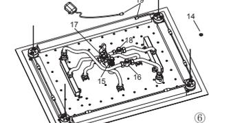
Before install the rainhead(9), install regulator(14) if needed. Remove the shower connectors(15, 16), hoses and washers, install regulators as the figure shown. Reinstall the washers, hoses and shower connectors.
