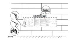
3 Mount the furniture on the steel plates and level the furniture by adjusting screws in anti-drop mounting bracket. Check the level using bubble level in-built inside the product.
