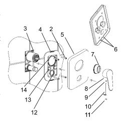
Install handle(8): Tighten the setscrew(9) with hex wrench(10). Press plug button(11) to the hole. The red part faces the left.
