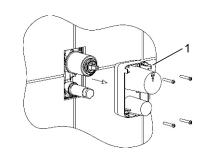
Slide the cover kit(4) onto the valve(3) with the plug(13) facing outside(**Note**: Don't squeeze out the rings12,14). Push it against the wall. Secure it with the screws(2, length 50mm). Slide the faceplate(5) onto the valve with slots(6) downwards, push it against the wall. Screw the bonnet(7) on the valve.
