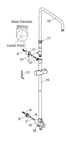
Remove and discard the guard from the tube kit(16), then install it into the slide bar kit. Install the nut(17) onto the tube kit with soft cloth between internal hole of the nut and the tube kit. Then screw the nut onto the slide bar kit with strap wrench or soft cloth between the nut and regular wrench.
