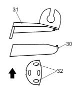
Replace bracket cover onto bracket base. Hang the handspray on the shower bracket.
