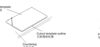
Trace the outline of the cutout template on the countertop with a pencil at the desired installation location. 用铅笔在厨房工作台面上您希望 安装水槽的位置画下切割模板的轮廓
