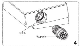
4. Install the assembly cartridge and stop in the body, adjust the stop pin into the notch.
