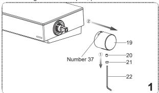
1. Before your action, make sure the number 37 on the temperature handle is upward vertically(It could not be turned counter-clockwise if not pushing the button). Remove the temperature handle(19).
