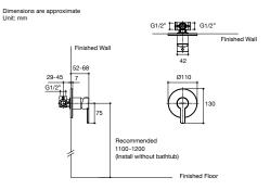
Note: The recommended dimension for installation can be adjusted according to user preferences and layout.
