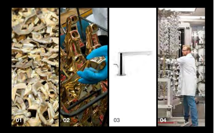
STEP Substrate and material (brass, zinc, etc.) is formed to make the faucets.
