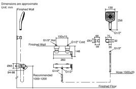
Jote: The recommended dimension for installation can be adjusted according to user preferences and layout
