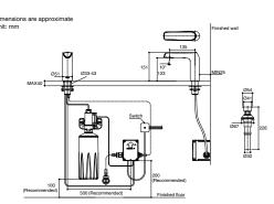
Note: The recommended dimension for installation can be adjusted according to user preferences and layout
