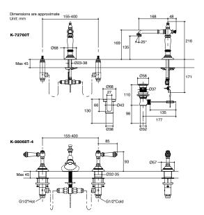
Note: The recommended dimension for installation can be adjusted according to user preferences and layout
