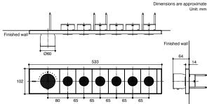
Note: The recommended dimension for installation can be adjusted according to user preferences and layout
