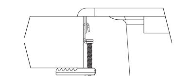
Paste sealing tape along the back rim of the sink.
