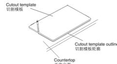
Trace the outline of the cutout template on the countertop with a pencil at the desired installation location. 用铅笔在厨房工作台面上您希望安装水槽的位置画下切割模板的轮廓。
