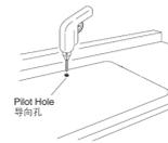
Cut along the outline to cut out the opening in the countertop 沿着画出的轮廓线切出水槽安装孔。
