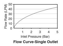
Note: 1. Flow rates are approximate. (1 gallon = 3.785 liters, 1 bar = 14.5 psi) 2. Dual outlet flow rate is higher than shown above but will vary.
