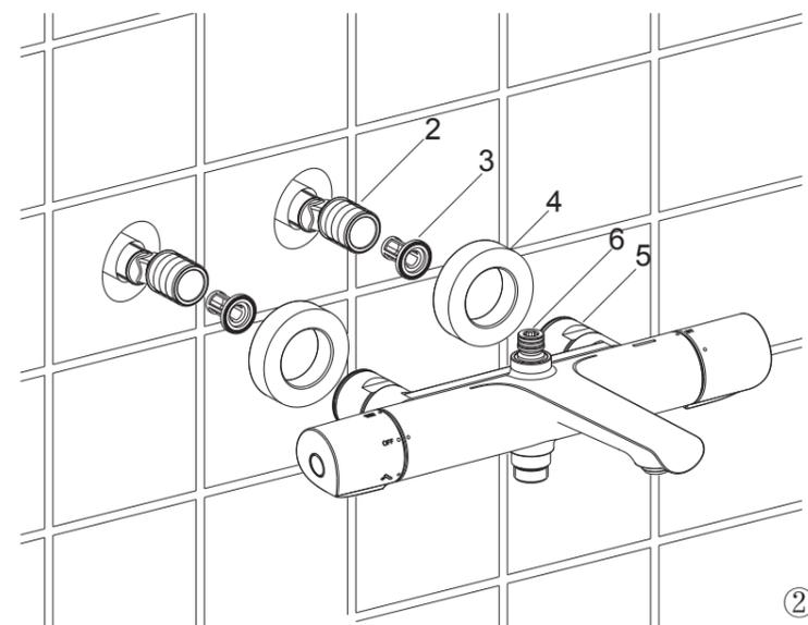
Put the filters(3) into the connectors. Slide the escutcheons(4) onto the faucet supply nuts(5).
