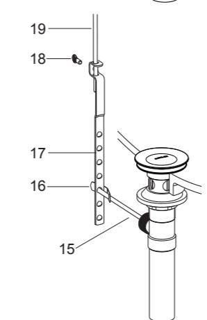
Assemble thumb screw(18) to link(17), and link onto ball lever(15) with 'V'-clip (16). Slide lift rod(19) in faucet and into the hole in link. Push the ball lever down into the open position, and adjust the lift rod. Tighten thumb screw(18).
