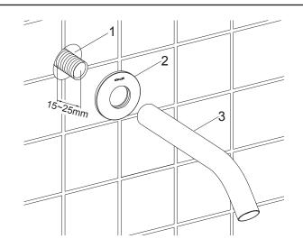
Apply tape or sealant to the G1/2" nipple(1, not provided) threads. Install the G1/2" nipple to extend 15-25mm beyond the finished wall.
