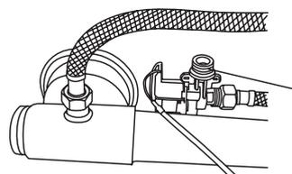
Inlet hole for the pipe cleaning inlet valve. Connect to cold water valve with hose.
