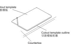
Trace the outline of the cutout template on the countertop with a pencil at the desired installation location. 用铅笔在厨房工作台面上您希望 安装水槽的位置画下切割模板的轮廓。
