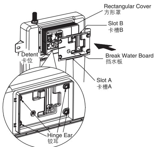
4. Insert the long screw through the hole on the break water board, and then tighten it.
