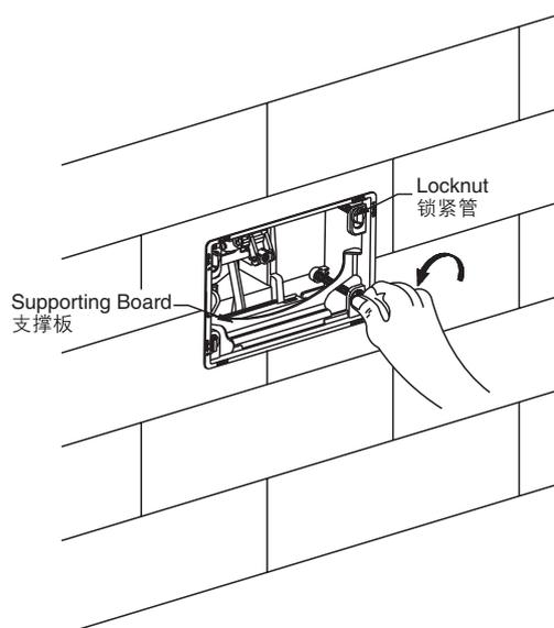
3. Tighten the long screws to the bolt through the hole.
