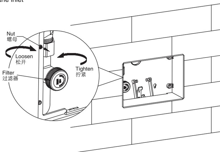
10. Loosen the filter nut as shown and take out the inlet valve to clean or adjust.
