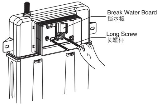
5. Screw the tightening screw to the "OPEN" position. Fix the supporting bracket in the arrow direction.
