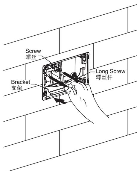
4. Install the cover as shown in the illustration. Put the lock on the cover directly on the reversed lock on supporting board, then push the cover and lock it. The installation shall begin from bottom to top.
