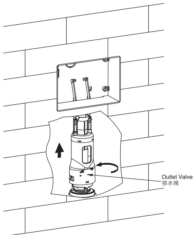
13. Take out the outlet valve as shown for cleaning or adjustment.
