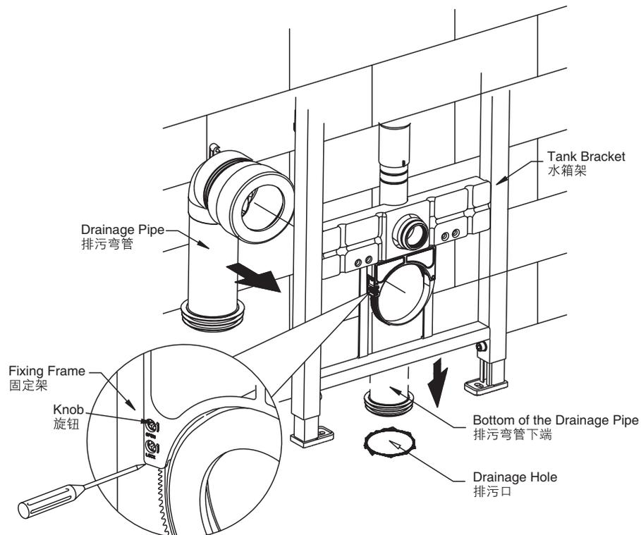
2. Tighten the long screw into the holes of the tank bracket and cover the drainage hole with the big filtration cap, cover the inlet hole with the small filtration cap.
