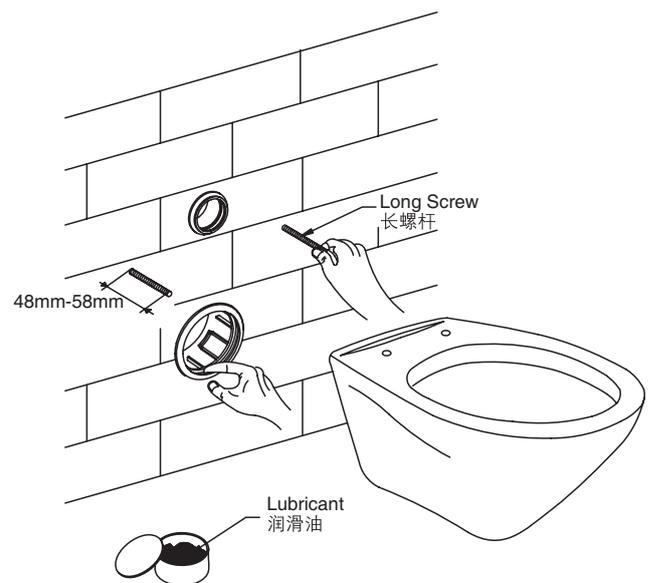
5. Install the toilet as shown in the illustration, and use a spirit level to ensure the lavatory to remain level.
