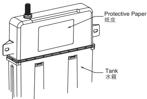
2. Fix the rectangular cover into the covering board of the tank. Tighten the four screws to firm the rectangular cover.
