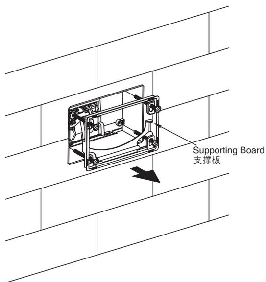
5. Take out the pole lock and the reversed lock as shown.
