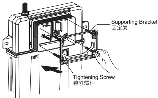
6. Adjust the supporting bracket to a proper position. Screw the tightening screw to the "CLOSE" position.
