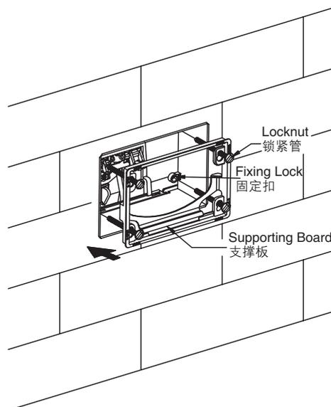
2. When fixing the supporting board, the locknuts should be screwed to the "LOCK" sign.
