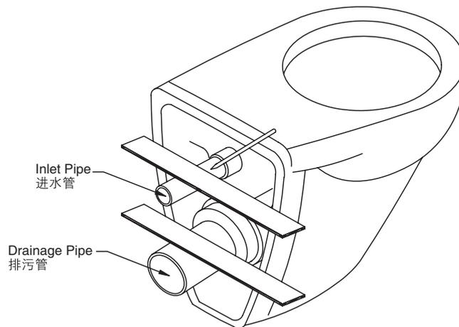
2. Eliminate unwanted part of the inlet pipe according to the marks of reserved space ,and rasp a smooth surface with files.
