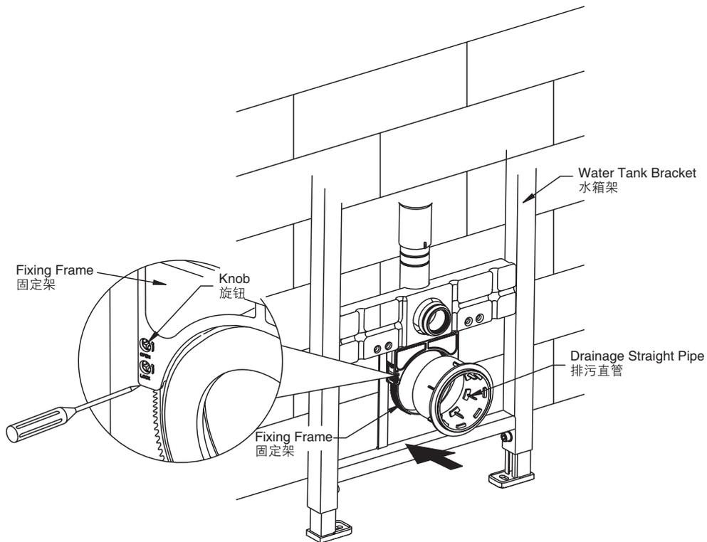
2. Tighten the long screw into the holes of the tank bracket and cover the drainage hole with the big filtration cap, cover the inlet hole with the small filtration cap.
