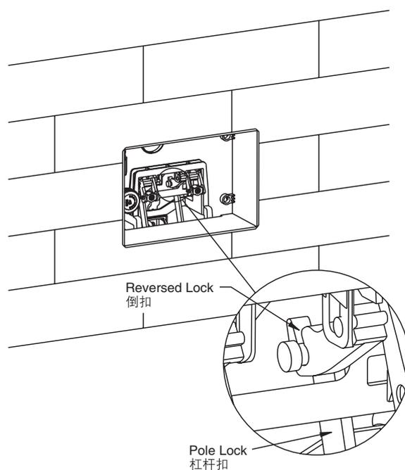
6. Hold the top of the bracket, and unplug the locknut by pulling the bracket.
