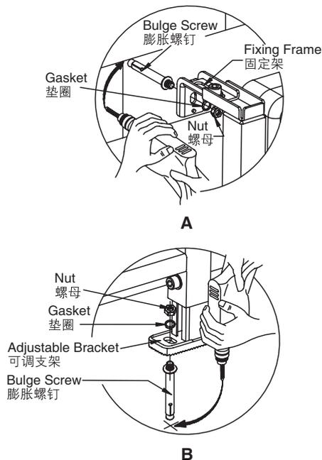
3. Tighten the nut with the spanner as shown in illustration A.
