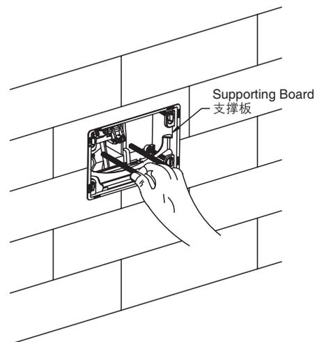
3. Tighten the locknut to the marked position of "OPEN" to take out the supporting board.
