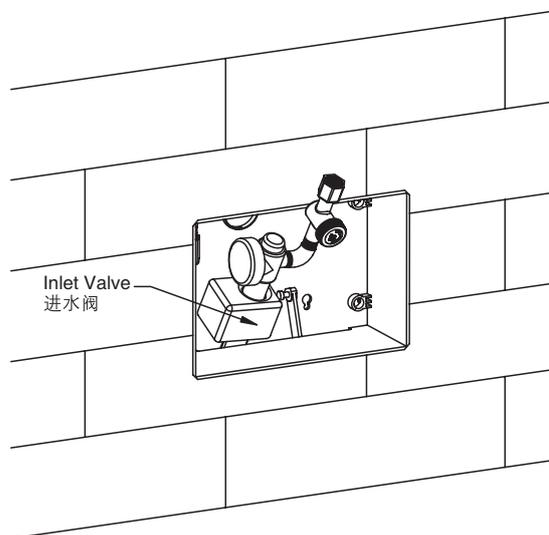
11. Hold the upside of the fixing lock, and take it out as shown.
