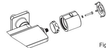
Unscrew the nut and stopper. Remove the cartridge cautiously. Clean the thermostatic cartridge by soaking it in warm vinegar.
