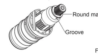
Install the bearing(without turning the spindle). Make sure the bulge of the bearing align with the groove of the body. Install the handle. Ensure the button on the temperature handle is upward horizontally and aligned with the faucet body. Tighten the screw with the washer. Install the handle plug.
