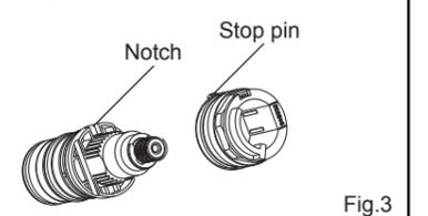
Install the assembly cartridge and stop in the body, adjusting the stop pin into the notch.
