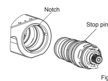
**NOTE:** Do not turn the cartridge when reinstall it. If you turned it without carefully, you should adjust it and be sure that the round mark is correctly in line with the groove, or readjust as per the steps of verification and setting.
