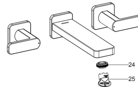
Ensure that all coupling nuts are tight. Ensure that the handles are in the off position. Turn on the main water supply and drain, and check for leaks. Repair as needed.
