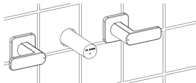
The figure shows the correct position of the handles when the installation is completed.
