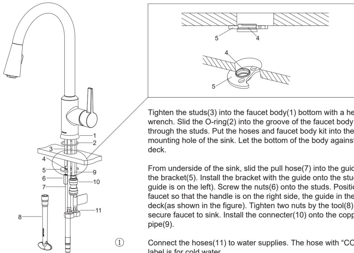
Tighten the studs(3) into the faucet body(1) bottom with a hex wrench. Slid the O-ring(2) into the groove of the faucet body through the studs. Put the hoses and faucet body kit into the mounting hole of the sink. Let the bottom of the body against the deck.
