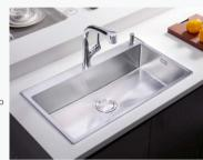
PURIST<sub>TM</sub> Large / Medium Self-Rimming Kitchen Sink K-45811T-2HD-NA Includes: Easy Clean Double Layers Duostrainer with Lid (114mm), Easy Clean Strainer (114mm), 50mm Anti-bacterial Trapway, Soap Dispenser, Stainless Steel Colander Dimensions: 840 x 470 x 200 mm
