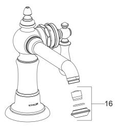
Ensure that all coupling nuts are tight. Ensure that the lever handle is in the off position.
