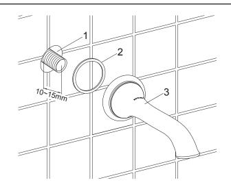
Apply tape or sealant to the G1/2" nipple(1, not provided) threads. Install the G1/2" nipple to extend 10~15mm beyond the finished wall.
