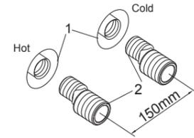
Flush the water supply pipes thoroughly to remove debris. Install the two offset connectors(2) into the hot and cold supply pipes. Use appropriate thread sealants or thread tape on pipe threads.
