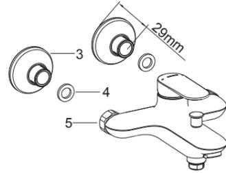
Put the washers(4) into the nuts(5), thread the nuts to connectors. Tighten the nuts with strap wrench or soft cloth between product and regular wrench.
