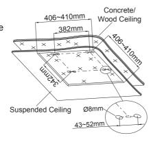
Make sure the end(3) of the stainless wire(1) is in the fix base(2) before install as shown to the right.
