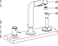
Ensure that all coupling nuts are tight. Ensure that the handle is in the off position. Turn on the main water supply and drain, and check for leaks. Repair as needed.
