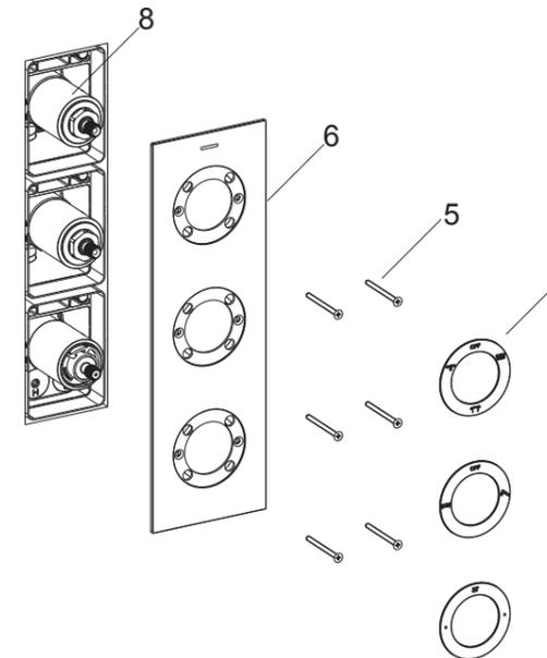
Before install the panel(6), take off the magnetic icon rings(7) from the panel.
