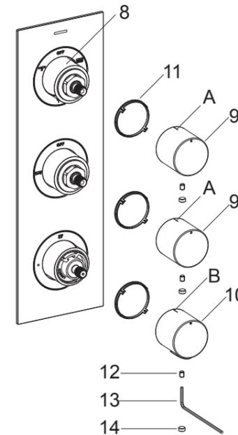
Install the handle kits(9,10) with washers(11) to the valves. Make sure the mark B of the handle(10) align to the number 37, the marks A of the handles(9) align to mark "OFF".
