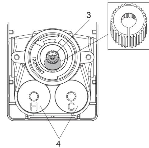
**NOTE:** Don't turn the cartridge spindle during the installation. Ensure that the notch of adapter(3) is downward.
