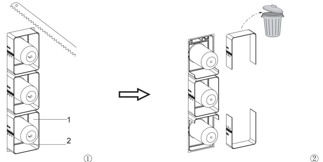
Cut the protrudent part from the side to the middle of the plastic guard(1) out of the finished wall. **NOTE:** Don't damage the valve guard(2).
