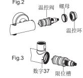
Clean the thermostatic cartridge by soaking it in warm vinegar. After that, install the cartridge back to the faucet body, aligning the notch with number 37(Fig.3). Tighten the nut and install stopper, keep the bulge side of stopper facing front and align it with number 37 as shown(Fig.4).
