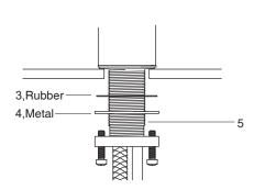
3. Slide the washers(3,4) onto the shank(5) and thread the ring onto the shank.
