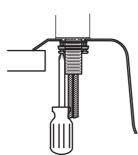
4. Tighten the screws to fix the faucet.
