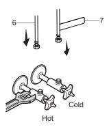
5. Connect the hoses(6) to water supplies. The hose with "COLD" label(7) should be connected to cold water supply.
