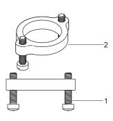
2. Partially thread the screws(1) into the ring(2).
