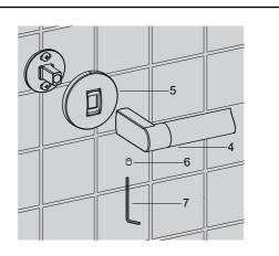
Slide the escutcheon(5) onto the bracket. Slide the main body(4) onto the bracket and keep the screw hole downward. Tighten the screw(6) with the hex wrench(7).
