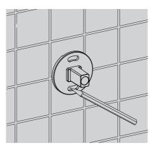
Select a location on the vertical wall to install the bracket. Mark anchor mounting hole location on wall as shown, ensure two screw holes of brack -et(3) are vertical. Drill hole in the finished wall as required.
