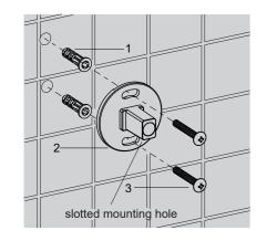
Press the anchor(1) into the hole. Orienting the slotted mounting hole of the bracket downward. Secure the bracket(2) with the self-tapping screw(3).
