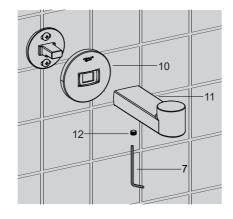
Slide the escutcheon(10) onto the bracket. Orient the "KOHLER" icon on escutcheon upward. Slide the main body(11) onto the bracket and keep the screw hole downward. Tighten the screw(12) with the hex wrench(7).
