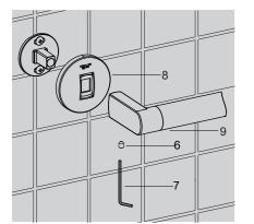
Slide the escutcheon(8) onto the bracket. Orient the "KOHLER" icon on escutcheon upward. Slide the main body(9) onto the bracket and keep the screw hole downward. Tighten the screw(6) with the hex wrench(7).
