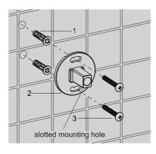
Press the anchor(1) into the hole. Orienting the slotted mounting hole of the bracket downward. Secure the bracket(2) with the self-tapping screw(3).
