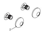
Thread the trim caps(2) onto the connectors until they contact the finished wall.
