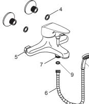
Insert washer seals(4) into supply nuts(5) of the faucets. Thread the faucet supply nuts onto the connectors and tighten.
