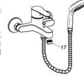
Ensure that all connections are tight. Ensure that the handle is in the off position.
