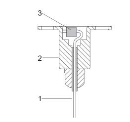
Make sure the end(3) of the stainless steel wire(1) is in the fixing base(2) before installation as shown in the figure.
