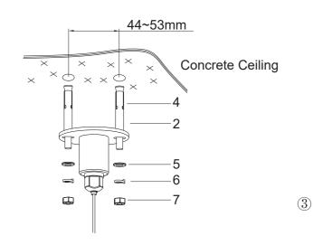
For concrete ceiling, drill 12 holes(Ø8mm) at the proper position in the concrete ceiling according to the marked dimensions and expansion screw's(4) diameter.
