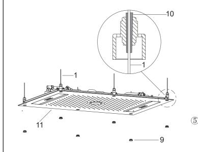
Flush the water supply pipes thoroughly for about one minute to remove debris. Gently pry the caps(9) from the shower head with a tool.
