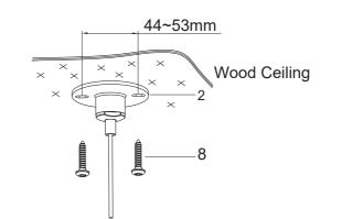
For wood ceiling, install each fixing base(2) along with a stainless steel wire with two screws(8) at the proper position in the ceiling according to the marked dimensions.
