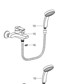
Ensure that all coupling nuts tightened.
